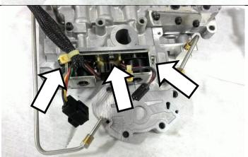
Place the aluminum solenoid block in place with the gasket below it.
