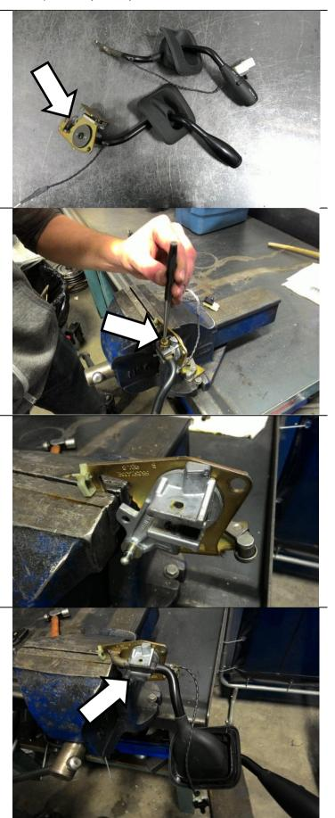
Reposition the spring and bushings for installation.
