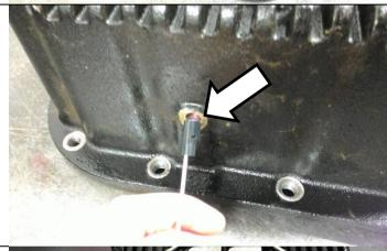
Apply thread sealant to the threads of the supplied harness/fitting and tighten it into the transmission pan.
