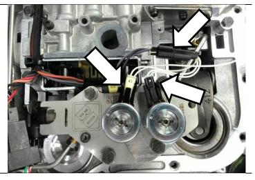
When you are finished this section, the transmission should have both solenoids connected. The loose single wire will be connected when the pan is reinstalled.
