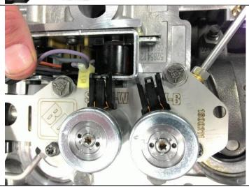
Connect the 1607254 solenoid harness (supplied with valve body) with the white plug going to the solenoid labelled SHIFT-W and the black plug going to GOV-B.
