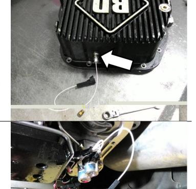
Raise the transmission pan below the transmission and connect the one pin connector from the governor solenoid wiring to the through pan wiring harness.
