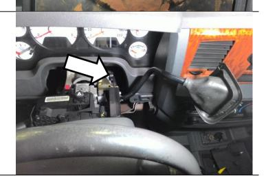
Follow the twisted black wire from the stock shift lever under the column to the two pin connector. Disconnect the plug and remove the push in retainer.
